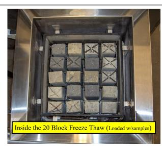
Our models hold from twenty (20) to eighty (80) 3" x 4" x 16" concrete test beams. However, specimen racks and cabinets can be customized to accommodate your needs.
